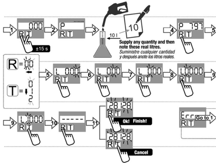
Press **TOTAL** and **RESET** (13 s). The display will show: 'P'. If it does not show 'P', it means that the meter is blocked. Call the **TECHNICAL SERVICE**.
